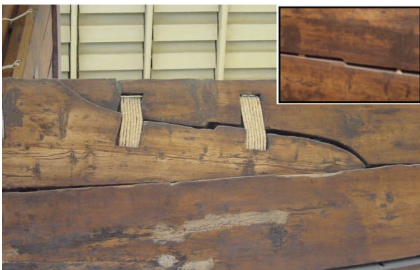
Fig. 2 Joggled scarf joint of Khufu I (author's photo); Inset: joggled strakes of Khufu I. (courtesy Paul Lipke Collection).
